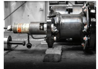
Replacing of spherical bearings
